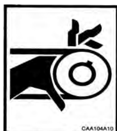
CAA104A10 Sheave/Sprocket Hazard
