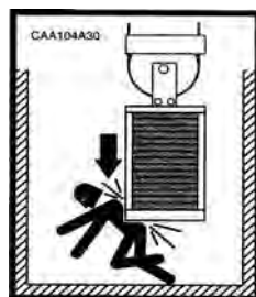
CAA104A30 Counterweight Hazard in Pit
