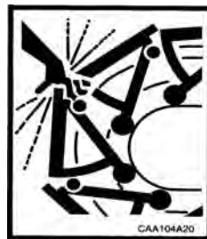
CAA104A20 Escalator Crush Hazard
