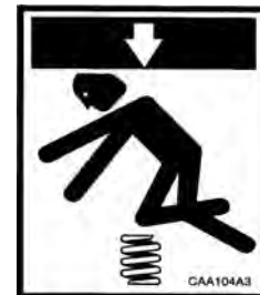
CAA104A3 Pit Crush Hazard
