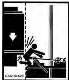
CAA104A28 Moving Equipment Hazard in Hoistway
