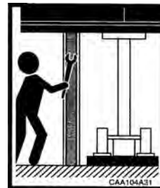
CAA104A31 Hydraulic Support Required When Working in Pit
