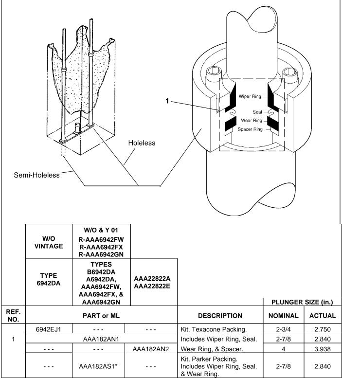
\* This kit is used where there is chronic leakage or noise that cannot be addressed with standard packing.
