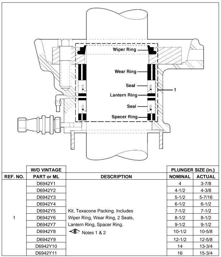
**NOTE 1:** These packing kits are for Otis "Cast Cylinder Head" designs made prior to 1974. **NOTE 2:** The spacer ring may be substituted with a lantern ring.
