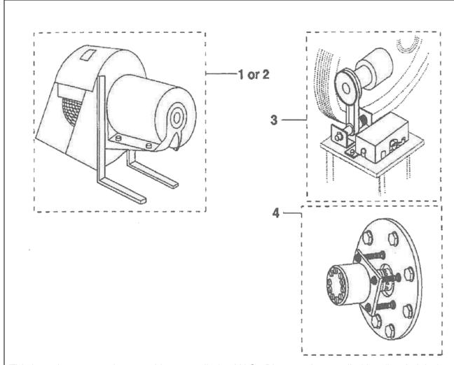
This item does not apply to machines supplied to NAO. Blower to be supplied locally. A right-hand blower unit is mounted on the right hand side of the machine when viewed from the commutator end. Left hand opposite.
