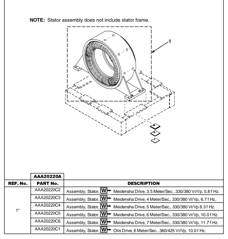
\* Reference number 1 is an item that would be refurbished. It is not cost effective to fabricate as new. Contact OSC or another competent motor rebuilding facility for refurbishment.
