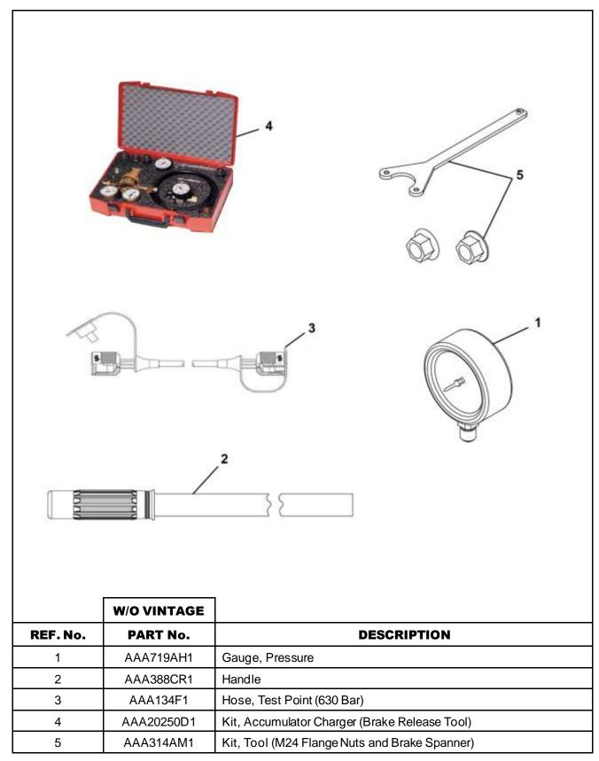
**NOTE:** These parts are used for brake release.
