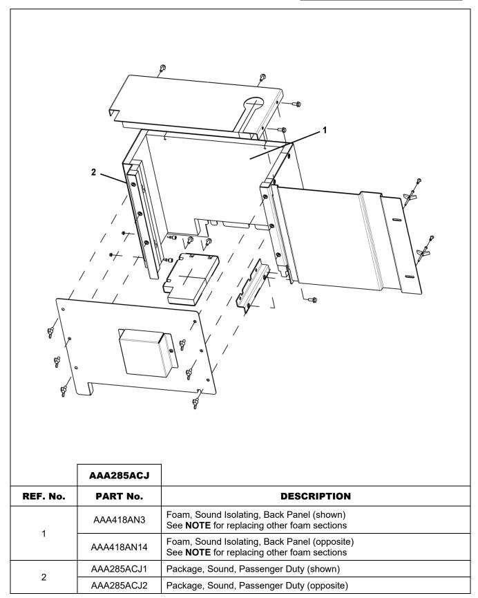
**NOTE:** To replace foam sections other than back panel, order ref. 2 and cut to fit on site.
