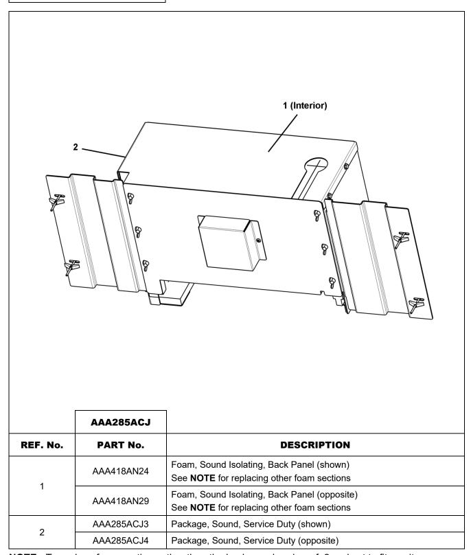
**NOTE:** To replace foam sections other than the back panel, order ref. 2 and cut to fit on site.
