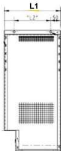
JAA384BDA1, L1= 250 mm JAA384BDA3, L1= 290 mm JAA384BDA2, L1= 250 mm JAA384BDA4, L1= 290 mm
