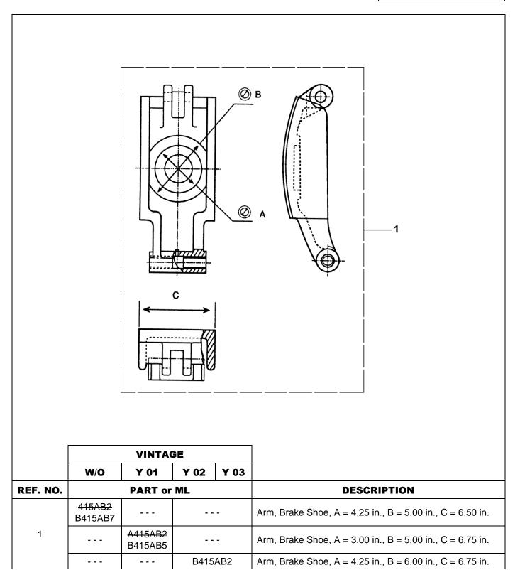
**NOTE:** All gearless machines must use brake arms that are lined with Green Gripper lining supplied factory-bonded by OSC. See TIP 6.0-1, *Replacement of Brake Linings*.
