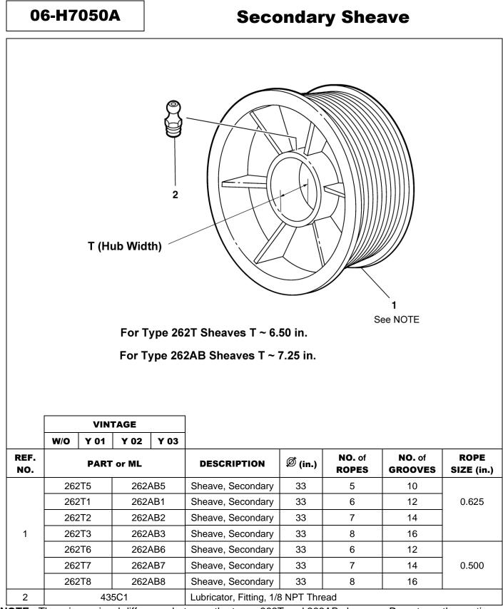
**NOTE:** There is no visual difference between the types 262T and 262AB sheaves. Do not use the casting number for identifying the sheave type. To identify the sheave, use sheave assemblies illustrations on pp. 13 and 14 and also hub width indicated above.
