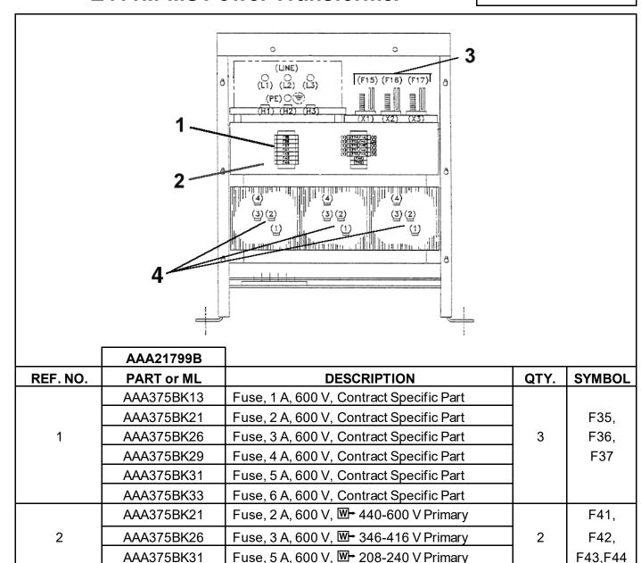
Fuse, Contract Specific Part, 250 V (provide current rating listed on fuse when ordering
