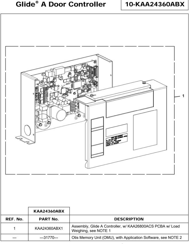
**NOTE 1**: This replaces the New Equipment version of the Glide<sup>®</sup> A controller box assembly with vintage tag 10-KAA24360ABG\_.
