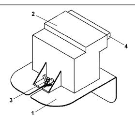
**NOTE:** Rope lubricator comes with a ground wire and must be grounded to function properly.
