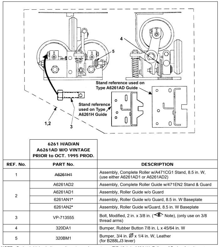
NOTE: Spring bridging bolts are alternate service parts per TIP 18.1-1, A6261H–Failure of Spring Attachment.
