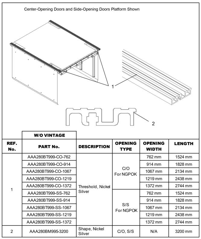
**NOTE:** Holes drilled in finished C/O and S/S thresholds are different, and parts are not interchangeable.
