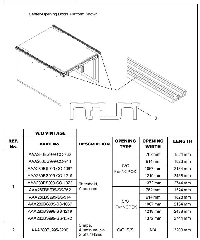
**NOTE:** Holes drilled in finished C/O and S/S thresholds are different, and parts are not interchangeable.
