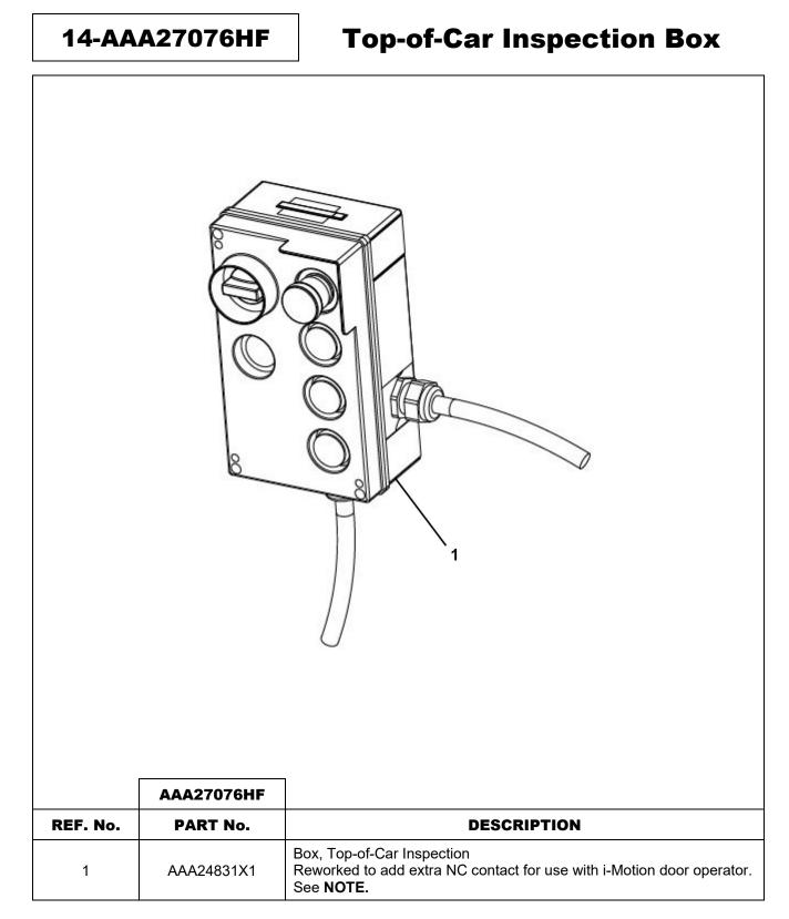
**NOTE:** Many Otis Americas TOCI box arrangements use Otis p/n DAA2431L002, which contains 3 NC contacts. The AAA24831X box contains 4 NC contacts, required with i-Motion door operators systems and other non-Otis designs that currently use all 3 NC contacts.
