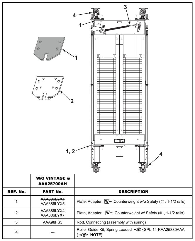
**NOTE:** To upgrade roller guide assemblies to spring loaded configuration, see TIP 18.1-8, *Roller Guide Selection and Sizing for Service and Modernization Applications.*
