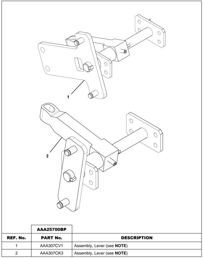
**NOTE:** Assembly includes one lever, one shaft, one key, and two pins.
