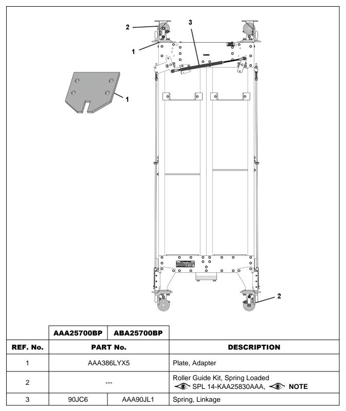
**NOTE:** To upgrade roller guide assemblies to spring loaded configuration, see TIP 18.1-8, *Roller Guide Selection and Sizing for Service and Modernization Applications.*
