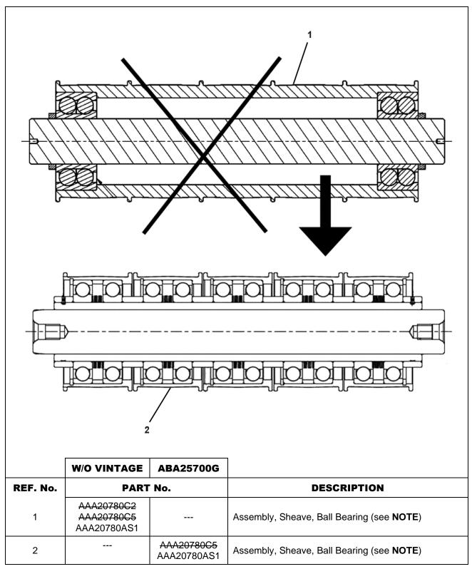
**NOTE:** Assembly includes one sheave, one shaft, and two spacers.
