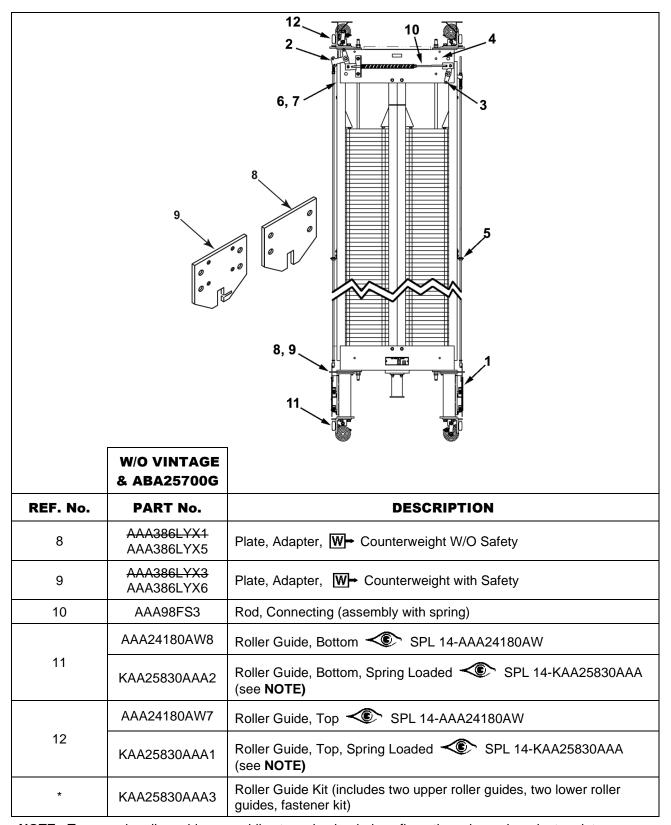
**NOTE:** To upgrade roller guide assemblies to spring loaded configuration, also order adapter plate.
