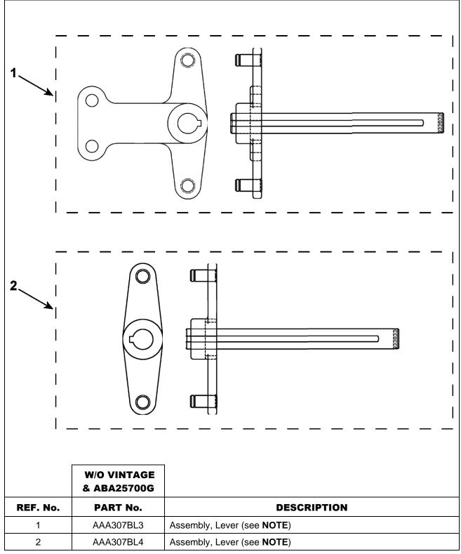
**NOTE:** Assembly includes one lever, one shaft, one key, and two pins.
