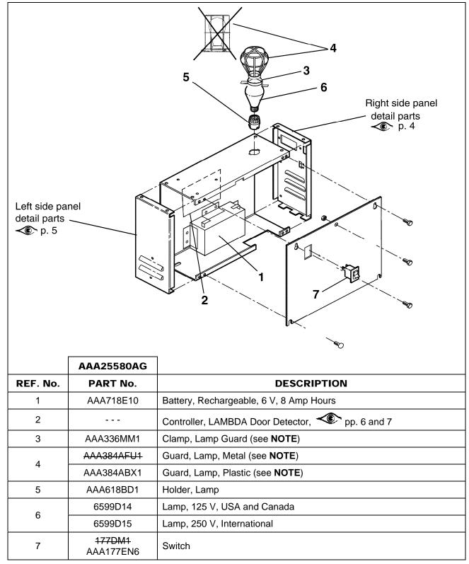
**NOTE:** Metal lamp guard p/n AAA384AFU1 is replaced with plastic guard p/n AAA384ABX1 and clamp p/n AAA336MM1.
