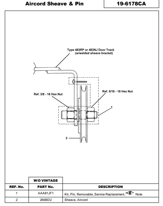
**NOTE:** Replaces pulley assembly on formerly welded bracket design when ordered w/ Ref. 2, TIP 21.2-5.
