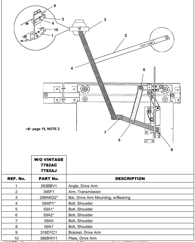
\*NOTE: Parts marked with \* are part of QL operator retrofit kit A7782AA500.
