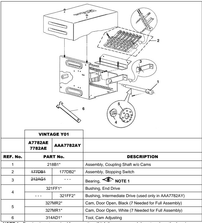
**NOTE 1:** Bearing is not required for operation. If it fails, remove and do not replace the bearing. However, retain the existing support bracket as box stiffener. New cam pack assembly uses a standoff as the box stiffener, taking place of the drive shaft support bracket with bearing.
