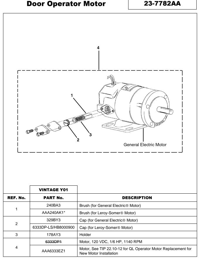
**NOTE:** Parts marked with \* are part of QL operator retrofit kit A7782AA500.
