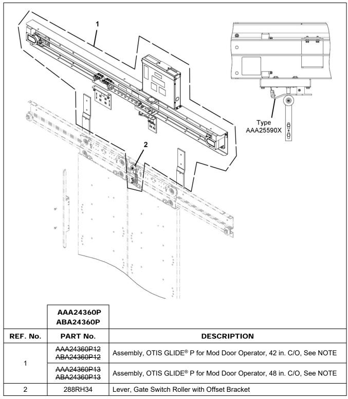
**NOTE:** OTIS GLIDE® P operators with AAA25590X style gate switch are no longer available, see TIP 22.17-5, OTIS GLIDE® P for Mod and Open Order Engine Unit Replacement.
