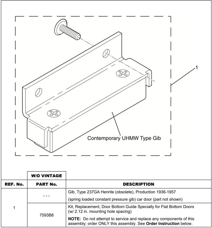
**Order Instruction:** It is recommended that door retainers be added to each door panel when installing new door guide kit 7593B8. Please order (2) AAA385RF3 and (6) AAA124FS3 per door panel onto which this replacement guide will be installed.
