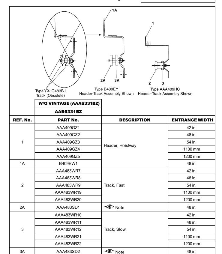
NOTE: When replacing type YXJO483BJ track, use ref. 2A & 3A and also ref. 5 & 6 from p. 4.
