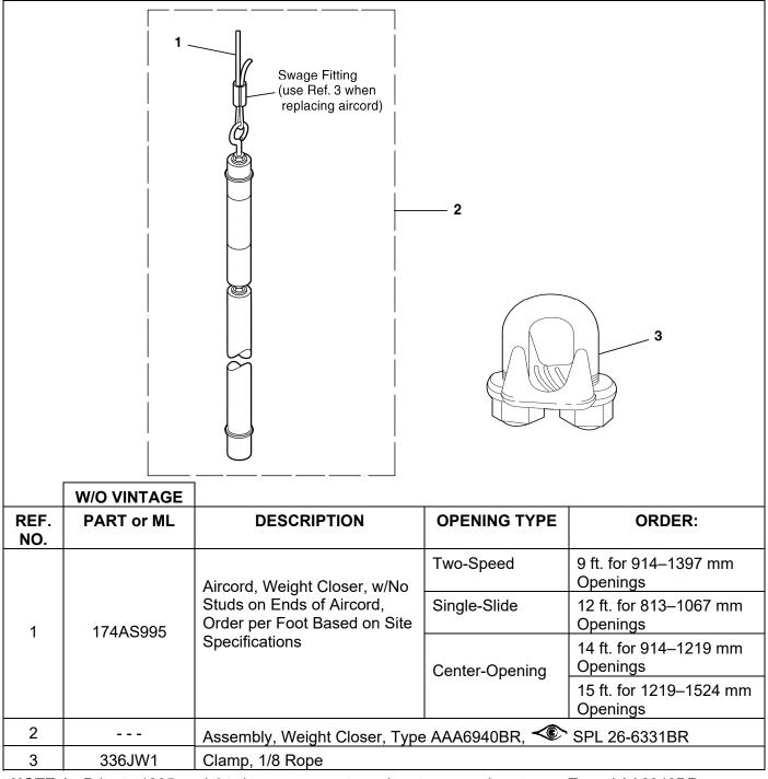
NOTE 1: Prior to 1995, weight closers were not used on two-speed systems. Type AAA6940BR was only used between September of 1995 and May of 1997. For subsequent closers
