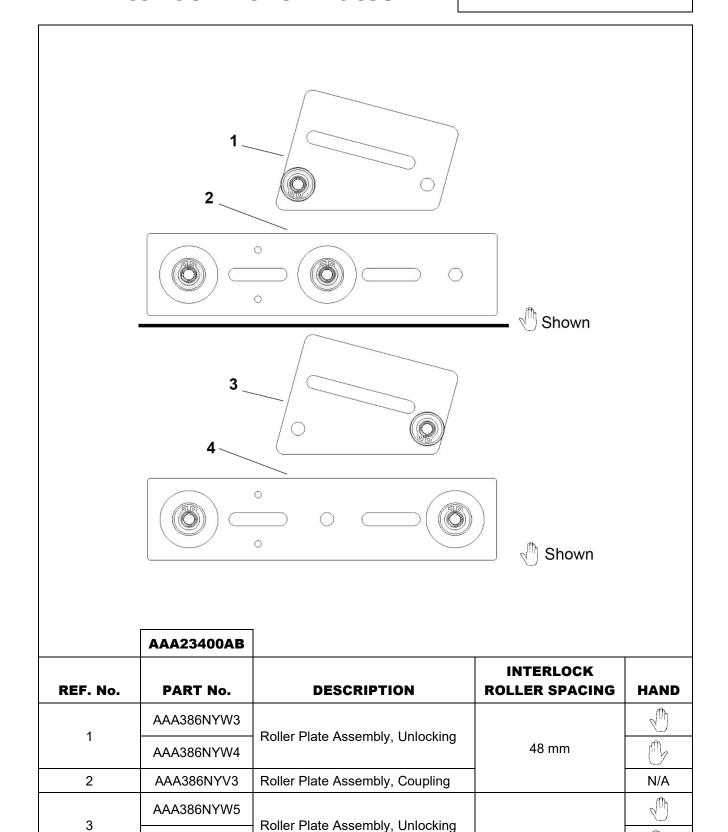
Roller Plate Assembly, Coupling
