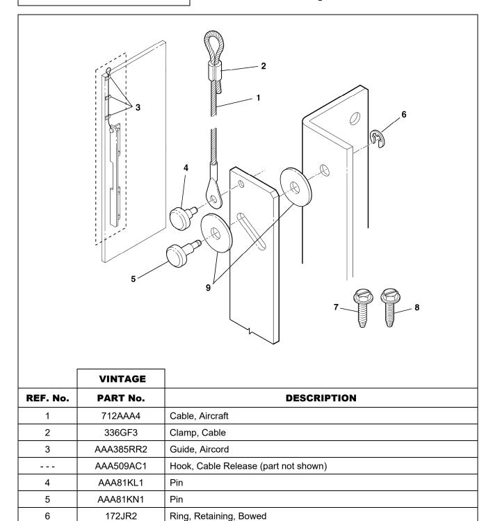
Screw, Thread-Forming 1/4-20 x 5/8 (for restrictor mounting)
