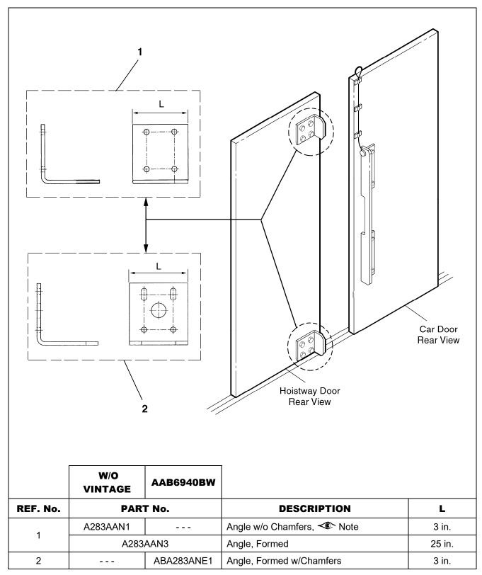
**NOTE:** It is highly advised that if the required maximum distances traveled outside of door zone are met by using the ref. 2 chamfered angle, you should order p/n AAA283ANE1. Check code and application and order accordingly.
