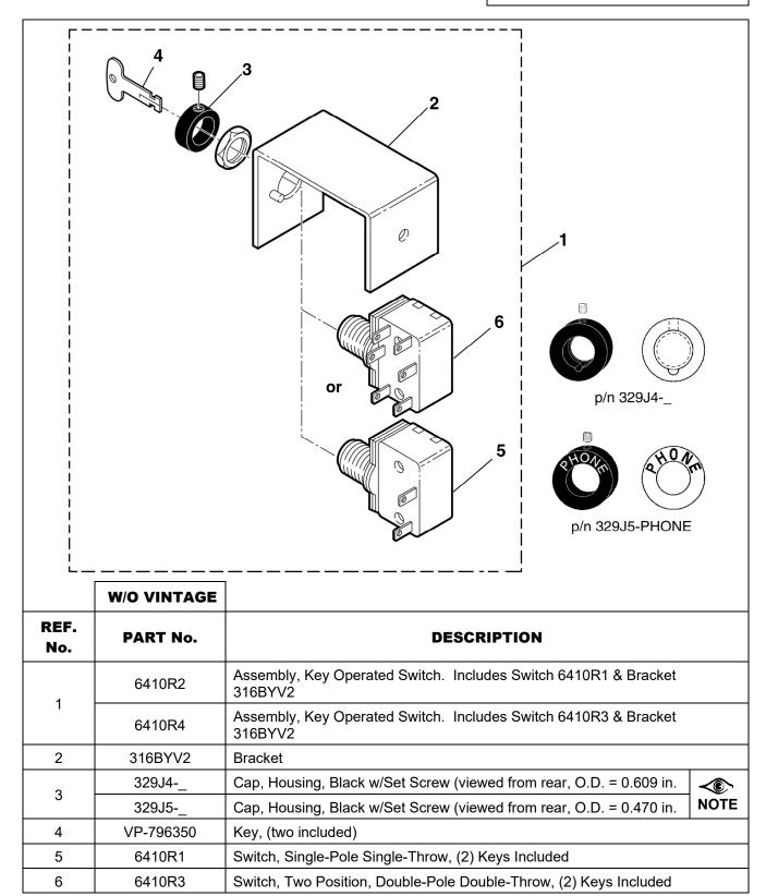
**NOTE:** Order a housing cap by indicating the desired marking after the dash:
