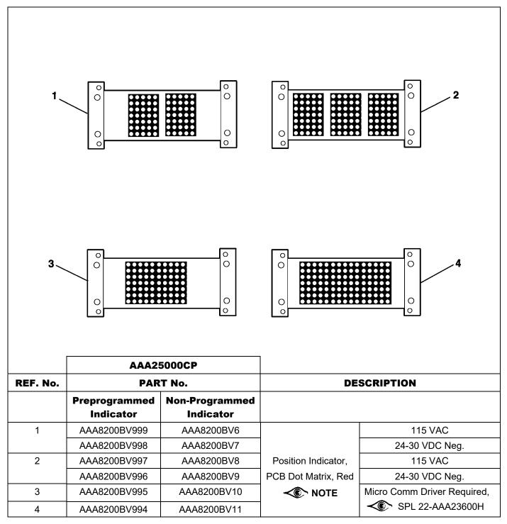
**NOTE:** Position indicators AAA8200BV6-11 are furnished with an EEPROM that is programmed with the building-specific floor markings. When ordering a replacement indicator, select 1 or 2 below.
