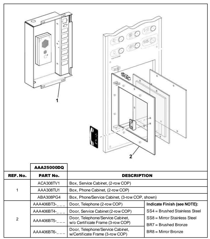
NOTE: When placing an order, add material finish to the part number, for example: AAA406BT3-SS4
