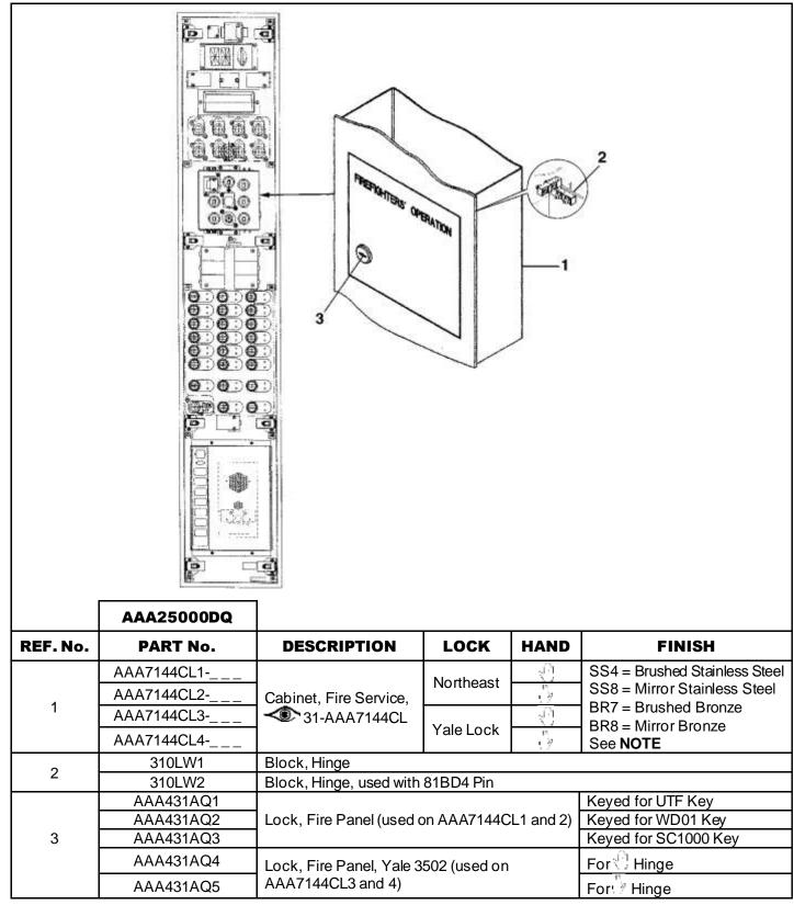
NOTE: When placing an order, add material finish to the part number, for example: AAA7144CL1-SS4
