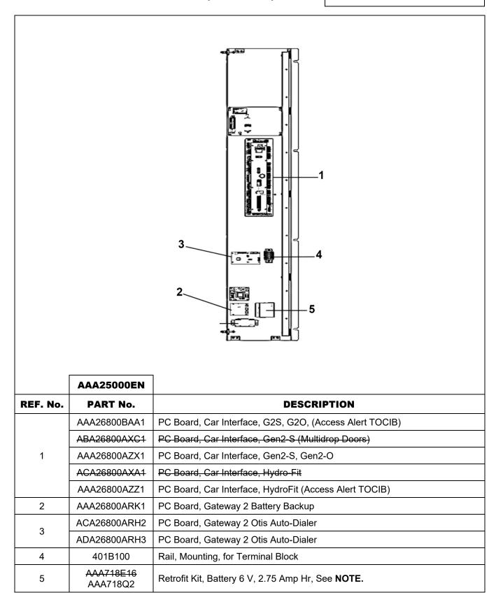
**NOTE:** AAA718Q2 is a retrofit kit. For more information, see TIP 20.2-5, COP Emergency Light Battery and Bracket Retrofit Kit Installation Information. Retrofit kit only needed if the AAA718E16 battery was existing equipment at the time of service, otherwise, replace with currently installed equipment.
