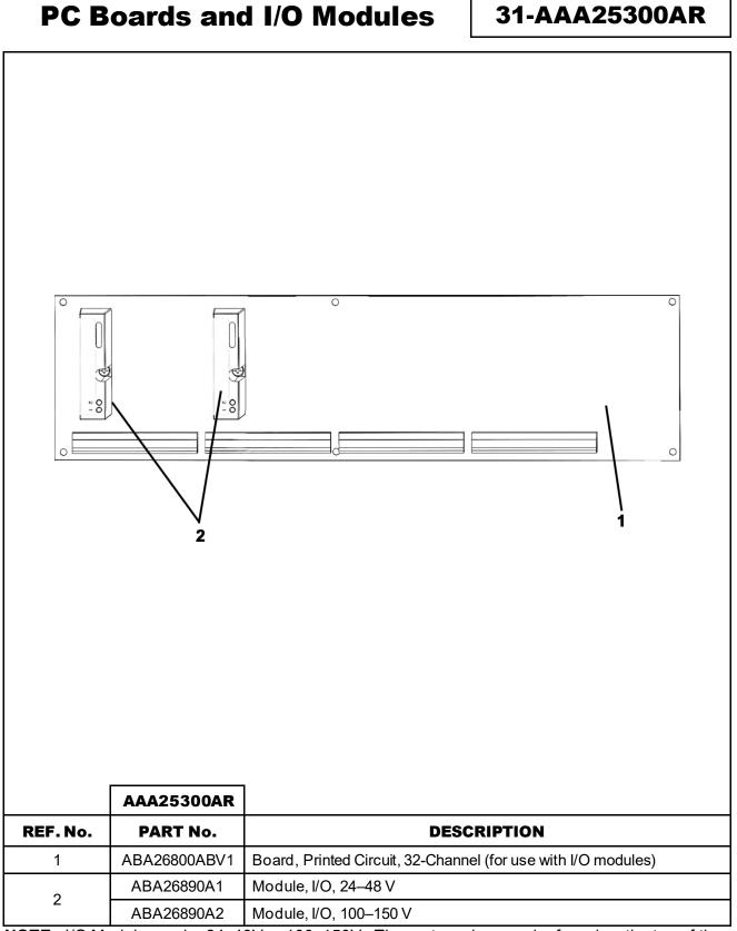
**NOTE:** I/O Module may be 24–48V or 100–150V. The part number may be found on the top of the module. Replacement of modules should be of the same type only, otherwise damage may occur.
