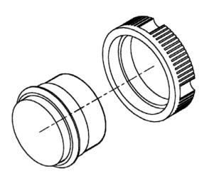
**NOTE:** All pushbuttons are 24 V with AMP connectors.
