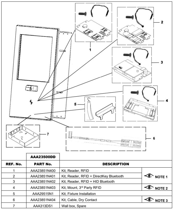
**NOTE 1: Kit includes:** RFID reader PCB, cable, and (4) M2X5 cross recessed countersunk flat head screws.
