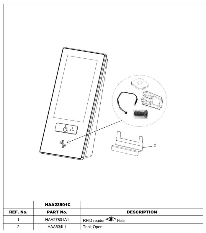
**NOTE:** Kit = RFID reader PCB + cable + (4) M2X5 Cross recessed countersunk flat head screws+ off-board LED.
