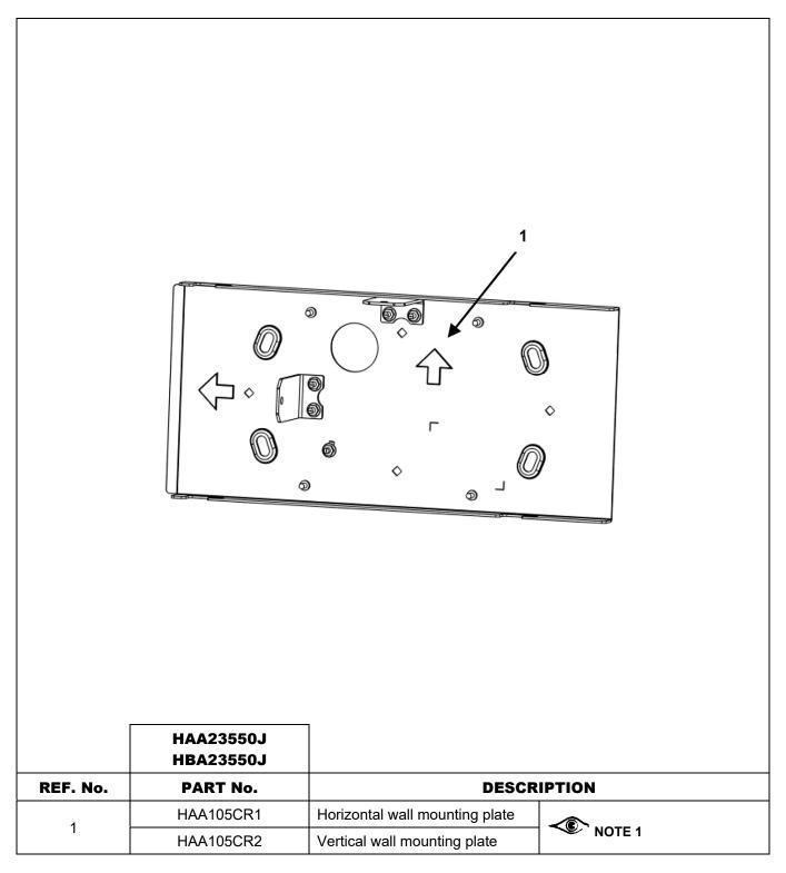
**NOTE 1:** Horizontal wall mounting plate recommended to be mounted above the hoistway door; vertical wall mounting plate recommended to be mounted on the side of the hoistway door.
