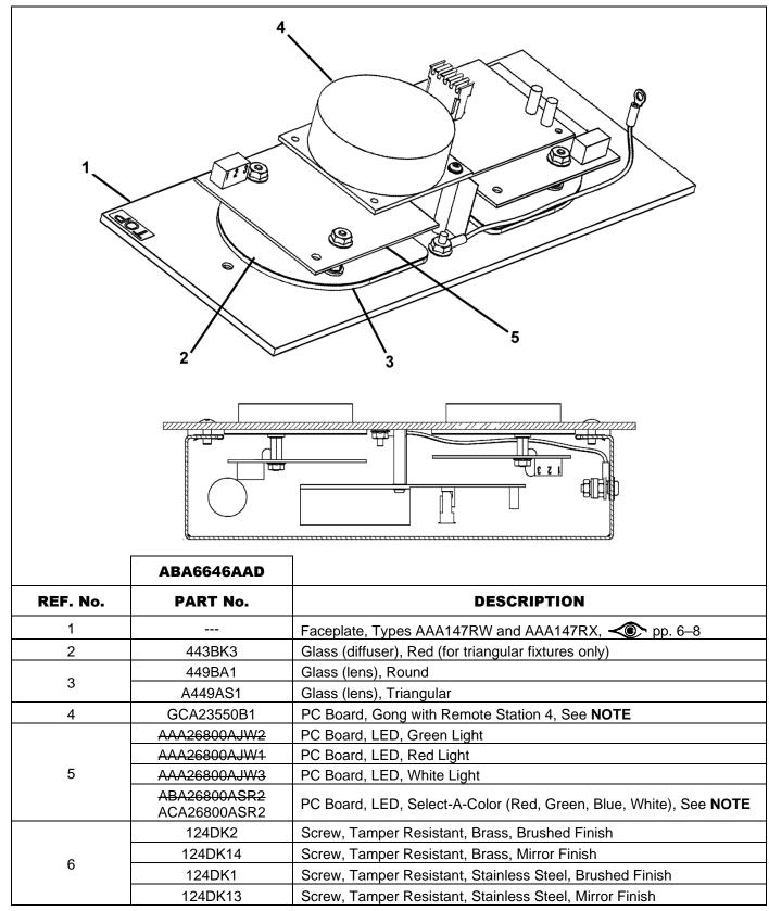
**NOTE:** The parts are available until stock is depleted. Once depleted, order p/n AAA26800BCD1 (dual LED) or p/n AAA26800BCM1 (single LED) PCB and p/n AAA174YL24 cable. See TIP 4.0-40 for replacement.
