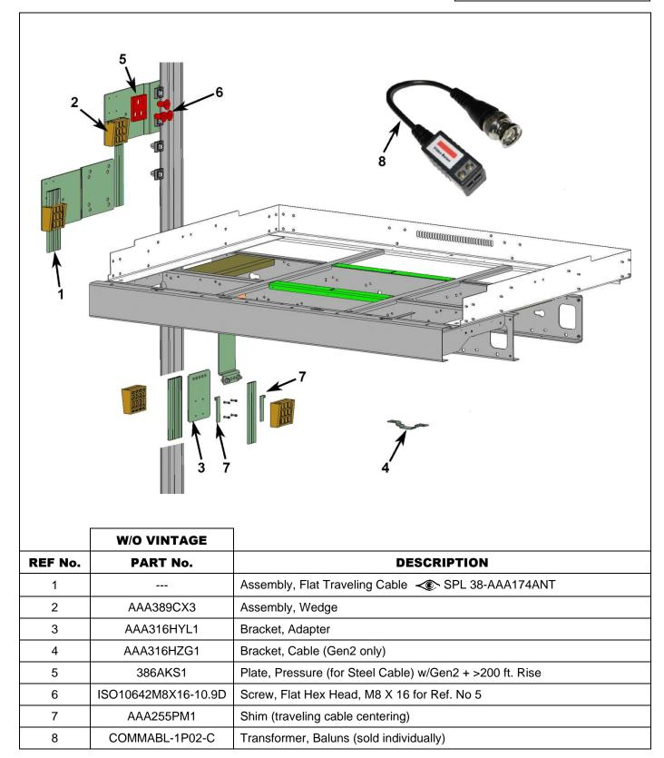
**NOTE:** Baluns transformers convert CAT5 video signal to twisted pair. One Baluns is required on each end of traveling cable.
