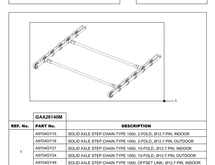
SOLID AXLE STEP CHAIN TYPE 1000, OFFSET LINK, Ø12.7 PIN, OUTDOOR
