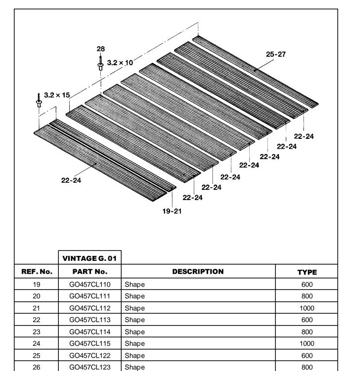
Blind Rivet 3.2x10, 3.2x15 Fastening Parts
