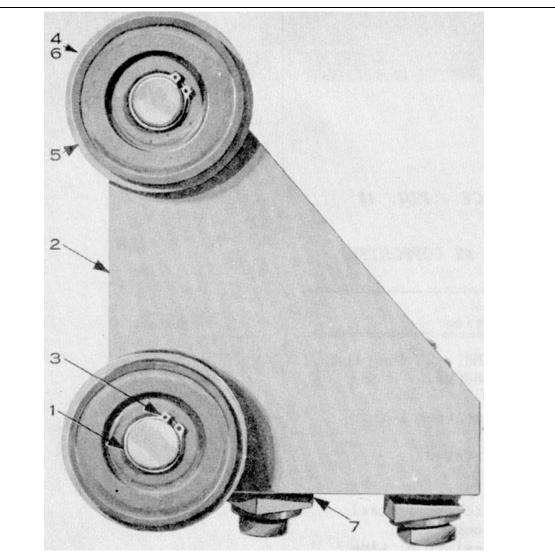
**Note:** Track (Guides) 483EV1, 483EW1, and 483EW2, shown on Page 12, were not furnished and cannot be used on tension carriage made to ML 6814B2 or ML 6814B3 (prior to 1951). These carriages were originally furnished without lower guides and with roller guides as shown above. Some of these roller guides have been replaced in the field by nylon step chain guides.
