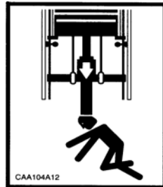
CAA104A12 Counterweight Hazard
