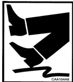
CAA104A8 Cord Hazard
