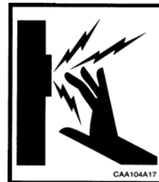
CAA104A17 Electric Shock Danger
