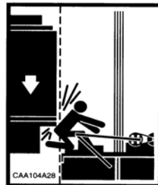
CAA104A28 Moving Equipment Hazard in Hoistway
