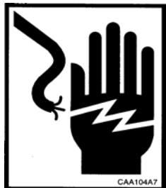
CAA104A7 Electric Shock Hazard
