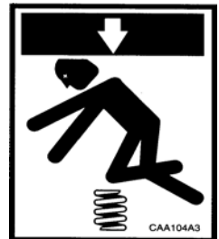
CAA104A3 Pit Crush Hazard
